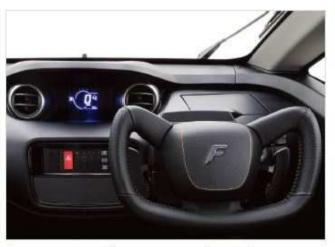
Steering accelerator is adopted to avoid breaking errors.
